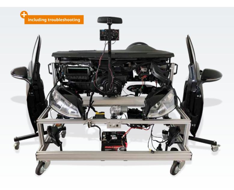
Experiments closely aligned to authentic practice using original components from a VW Golf 7, already based on Volkswagen's modular component matrix MQB. This networked systems training model focuses on an actual CAN gateway as well as the complete steering column electronics and encompasses a fully operable front door complete with comfort control system.
