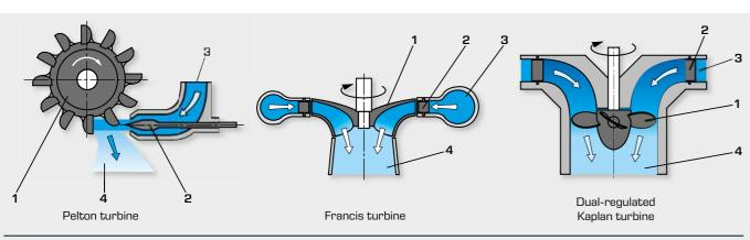
1 rotor, 2 distributor, 3 water inlet, 4 water outlet
