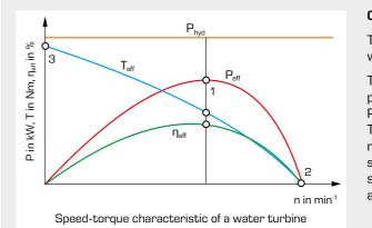
P<sub>hvd</sub> hydraulic input power of the turbine,
