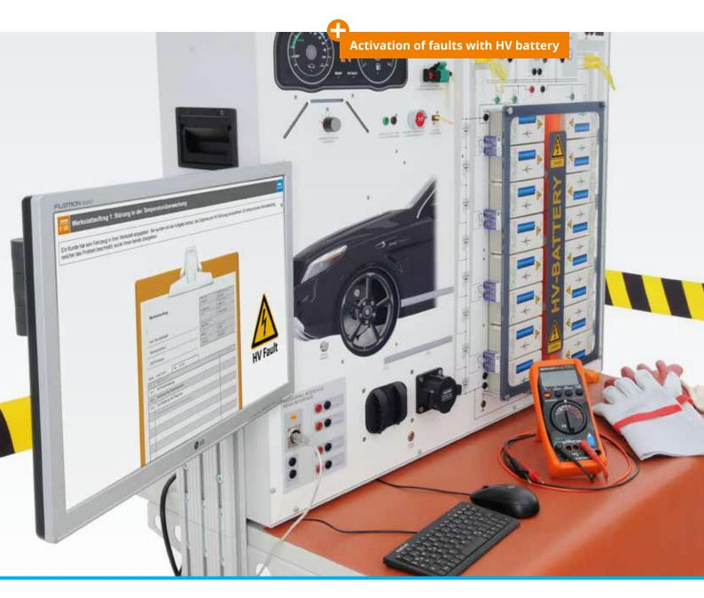
Diagnosis of faults which can be specifically activated allows students to gain skills which will be of use to them in a real vehicle workshop.
