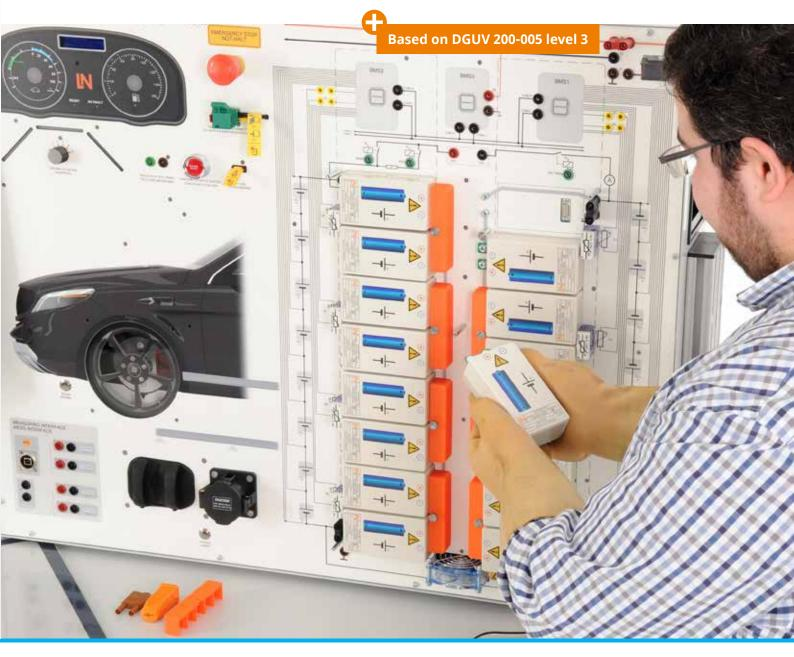
Working directly on a real high-voltage battery and inside it: The system is set up to be just like a high-voltage battery in a standard production vehicle. With this training system, trainees can make measurements and diagnoses inside the high-voltage battery, working down to the level of individual cells and even replacing them.
