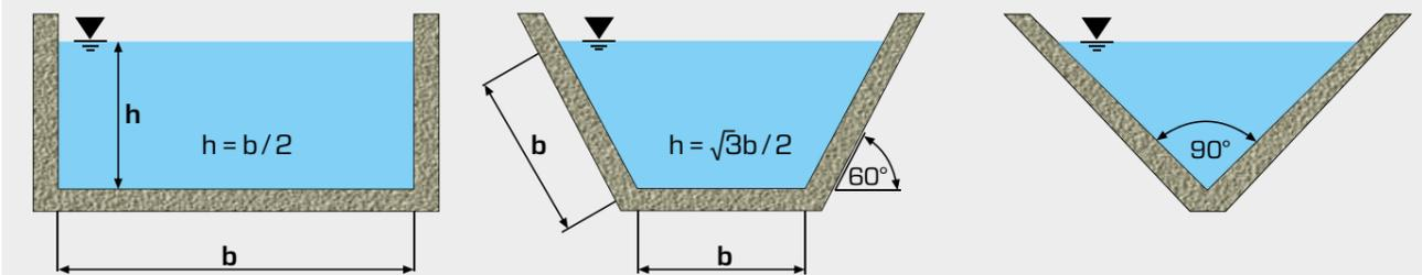
Rectangle, trapezoid with 60° angles, triangle;  $h$  discharge depth,  $b$  flume width
