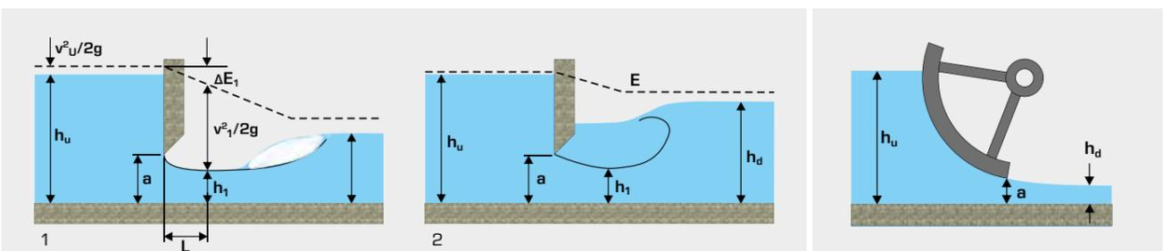
Discharge under a sluice gate
