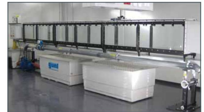
The largest GUNT experimental flume HM 161 – with a cross-section of 600x800mm and a 16m long experimental section – offers a large number of possibilities for your own research projects.
