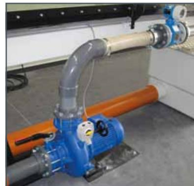
Pump (HM 162) with shut-off valve with manual actuation in the delivery side for adjusting the flow rate (above the pump). The pump's delivery line also contains the hose and the electromagnetic flow meter. The shut-off valve is only needed for wave experiments.
