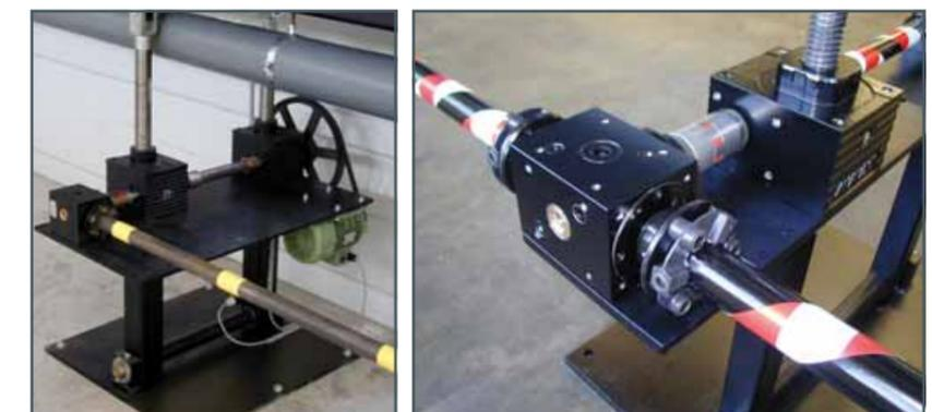
Electrical inclination adjustment in HM 161
