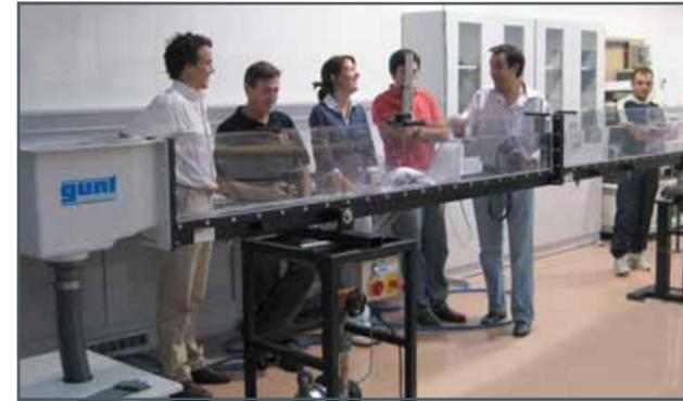
The HM 160 flume is perfectly suited as an introduction to the topic of open-channel flow and the demonstration of many of the basic principles. This flume is compact and required little space.
