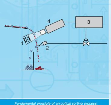
*1* light source, 2 compressed air jet *3* image analyser with controller *4* camera
