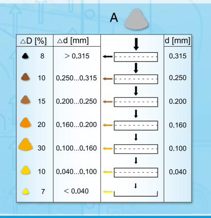
Classification of a feed (A) by sieving: d sieve mesh width,  $\triangle d$  particle size interval  $\triangle D$  proportion of particle size interval referred to feed
