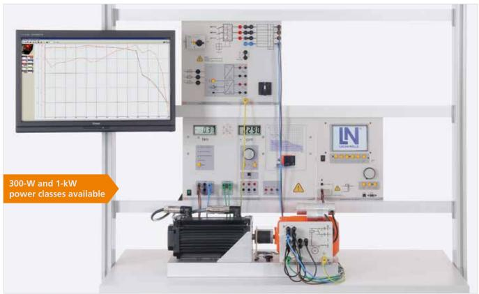
Experiment example: "Single-phase motor with operating and auxiliary capacitor EEM 3.4"
