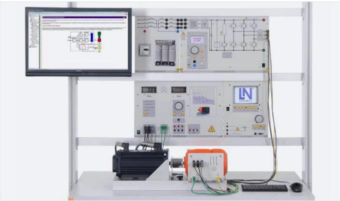
Training system: "Frequency converter drive with servo machine test stand"
