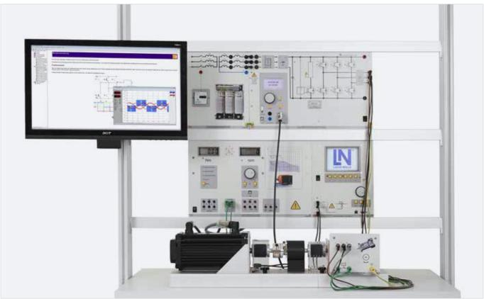
Training system: "Servo drives with a servo machine test stand"
