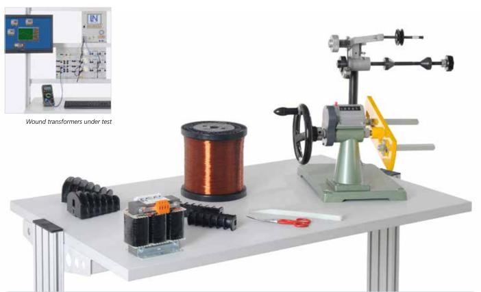
Experiment example: "Winding transformer coils EMW 10"
