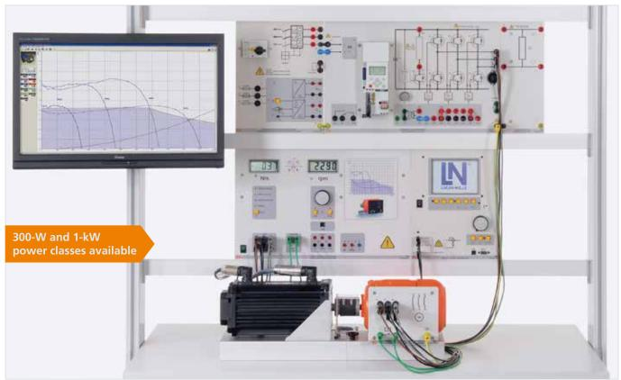
Experiment example: "Frequency converter drives EDT 25"
