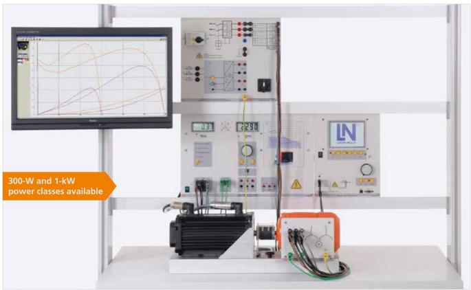
Experiment example: "Three-phase pole-switchable motor with two separate windings EEM 4.3"
