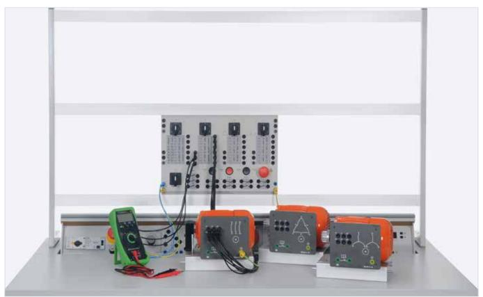
Experiment example: "Manual switching in three-phase circuits EST 1"
