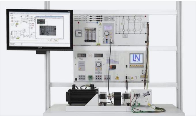
Training system: "Variable-speed permanent-magnet servo drives with Matlab®/Simulink® and the servo machine test stand"
