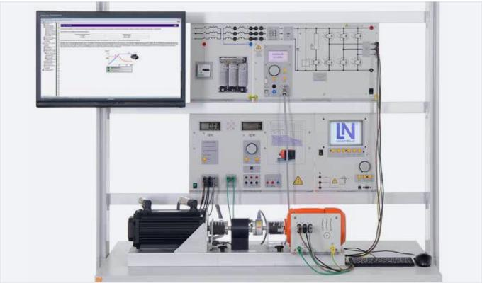
Training system: "Field-oriented control of asynchronous motors with Matlab®/Simulink® and a servo machine test stand"
