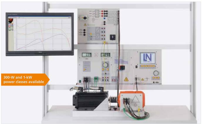
Experiment example: "Three-phase, pole-switchable motor according to Dahlander EEM 4.2"
