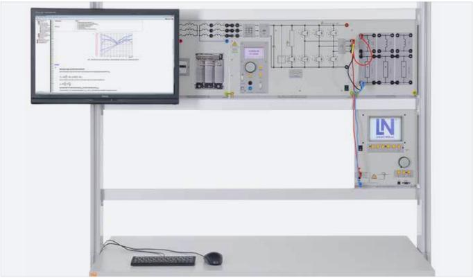
Training system: "Self-commutated power converter with a passive R-L load"
