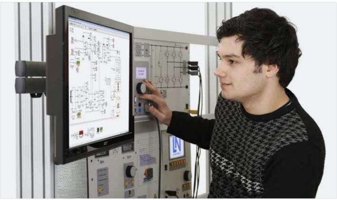
Training system: "Field-oriented control of asynchronous motors with Matlab®/Simulink®"
