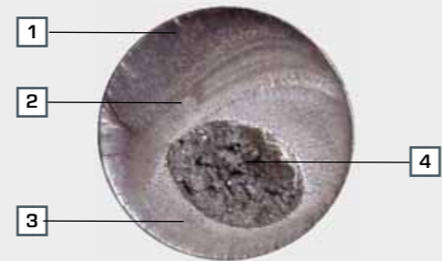
Analysis of the fracture surface following the fatigue strength test
