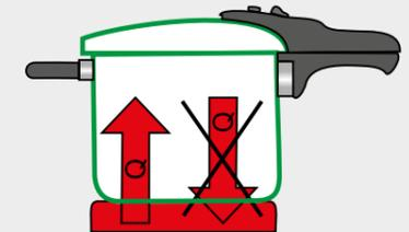
Referring to the example of the pressure cooker after the inside of the cooker has warmed up, the heat in the cooker cannot flow back into the heating plate.
