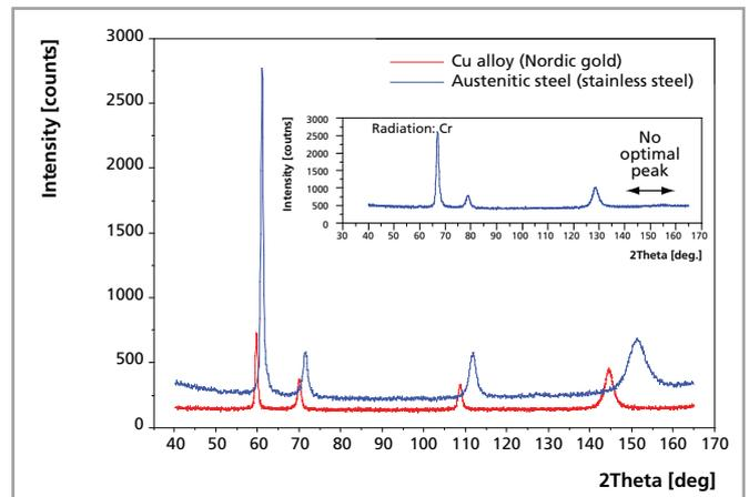
Reflections are in the desired range for these materials when using a Mn tube
