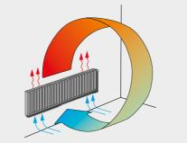
The air molecules warmed by the heater rise due to differences in density
