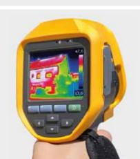
Using a thermal imaging camera, it is possible to make thermal radiation visible: the thermal camera converts long-wave infrared radiation into visible radiation.
