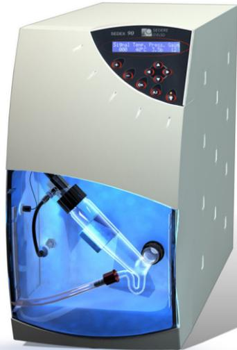
As an universal detector, an ELSD offers numerous possibilities for detecting substances that have few or no chromophores. Since the eluents are evaporated, the use of non-UV-compatible solvents poses no problems and the ELSD is gradient compatible.
