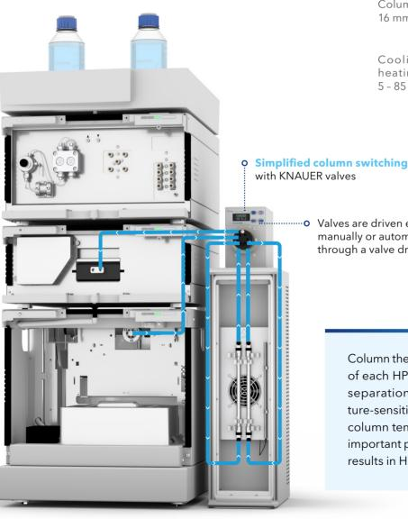
• Wide space. easy handling Up to 6 columns with maximum o 300 mm length Columns up to 16 mm ID Cooling and heating from o 5 - 85 °C
