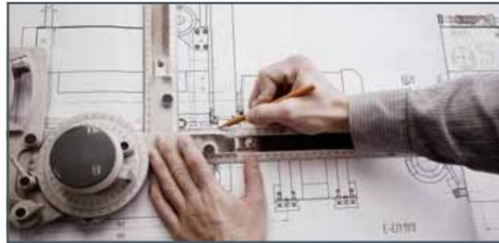
Engineering drawings present a very abstract image of the components or devices with precise specifications. Using geometric and graphical features such as lines and symbols, as well as alphanumeric characters such as digits and letters, a three-dimensional object is described in two dimensions.
