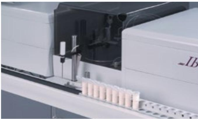
A stirrer mechanism, designed with the least possible carryover (a single point of contact) stirs and draws the sample to be tested. The autosampler is also equipped with a wash station to thoroughly clean the pipette (inside and out) with a cleaning solution after each sample. The carry-over typically around 0.25% fully complies with the ISO 16140 standard ( $\ll 1\%$ ).
