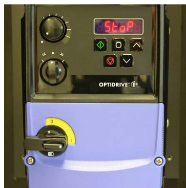
Fig. 8b Switch 1 set to ON
