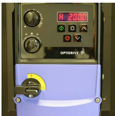
Fig. 8d Switch 3 set to 200 Hz
