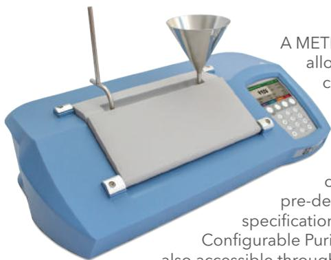
A METHODS system allows for quick configuration, with reading type (continuous or single-shot) and limit checking against pre-defined product specifications made simple. Configurable Purity equations are also accessible through the easy-to-use software using the keypad.
