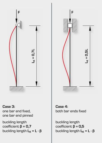
To determine the buckling stress we use the degree of slenderness  $\lambda$  as a material parameter and the moment of area radius i.
