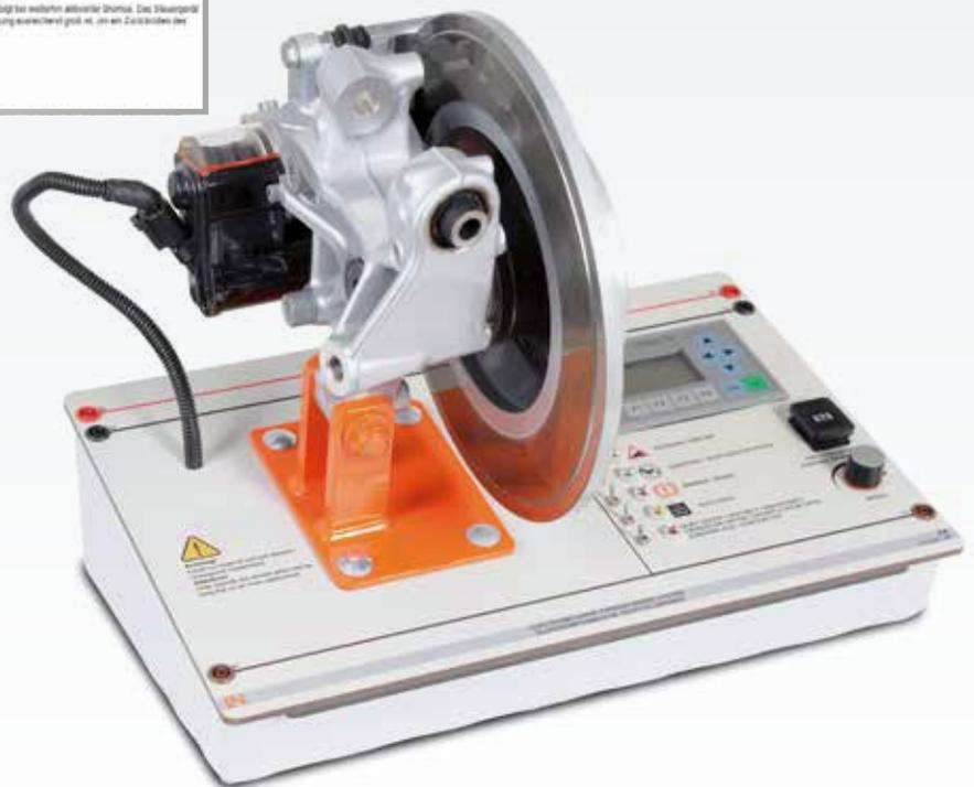
An electromechanical parking brake replaces the conventional handbrake with a simple switch on the dashboard. This means there is no need for a handbrake lever. The switch can activate the parking brake on the rear wheels with the aid of an electromechanical actuator.
