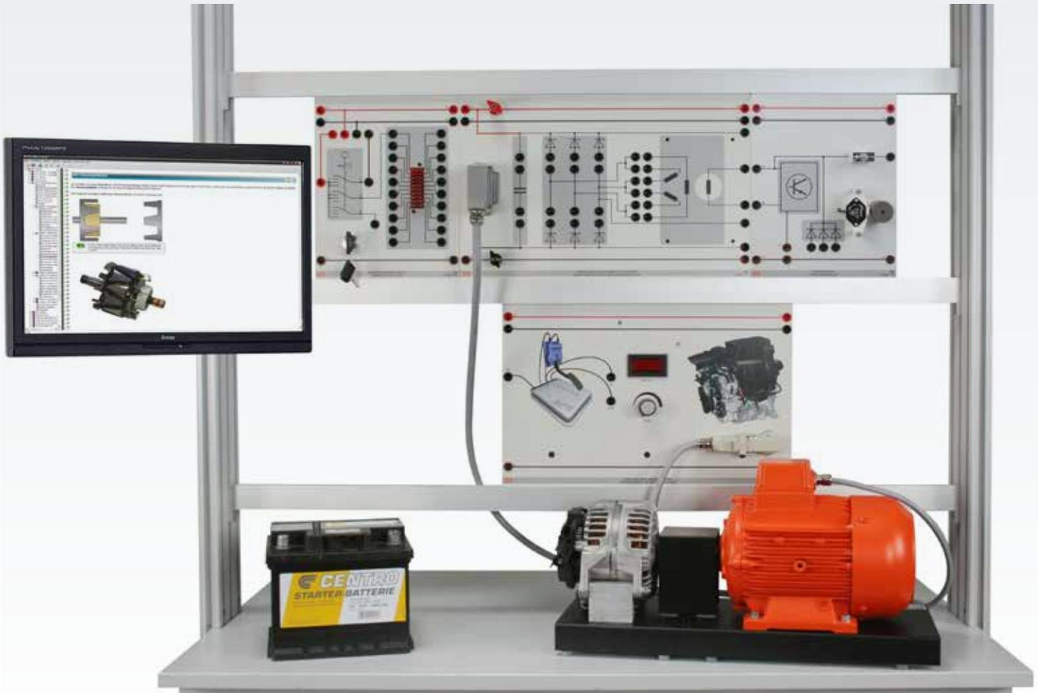
Our system enables trainees to become familiar with the function of a hybrid controller. They can experiment for themselves and observe how the voltage generated by an alternator is maintained at a given level at all engine revs and with any loading. The role of the average excitation current is explored as well as how changes are brought about in the magnetic field and stator winding induction.
