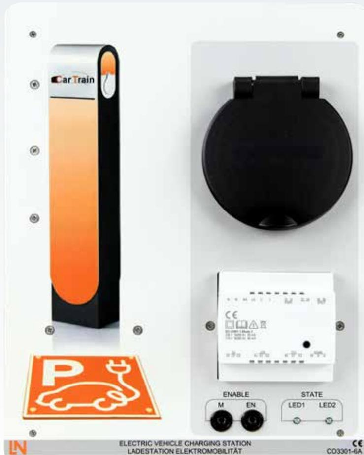
A real charging station: This training system provides an educationally modified version of an authentic charging station. In conjunction with the CarTrain electric vehicle set, it is possible to understand how communication between vehicles and charging stations proceeds.
