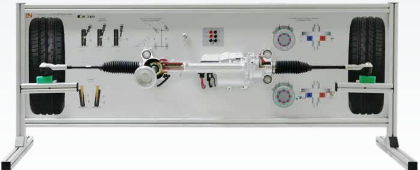
Electromechanical servo-steering offers many advantages over steering systems without such assistance. It provides not only physical, but also psychological benefits to drivers. Steering assistance is provided based on need. This means that it only becomes active when a driver wants it. Simultaneously, though, it also responds to speed, steering torque and angle.
