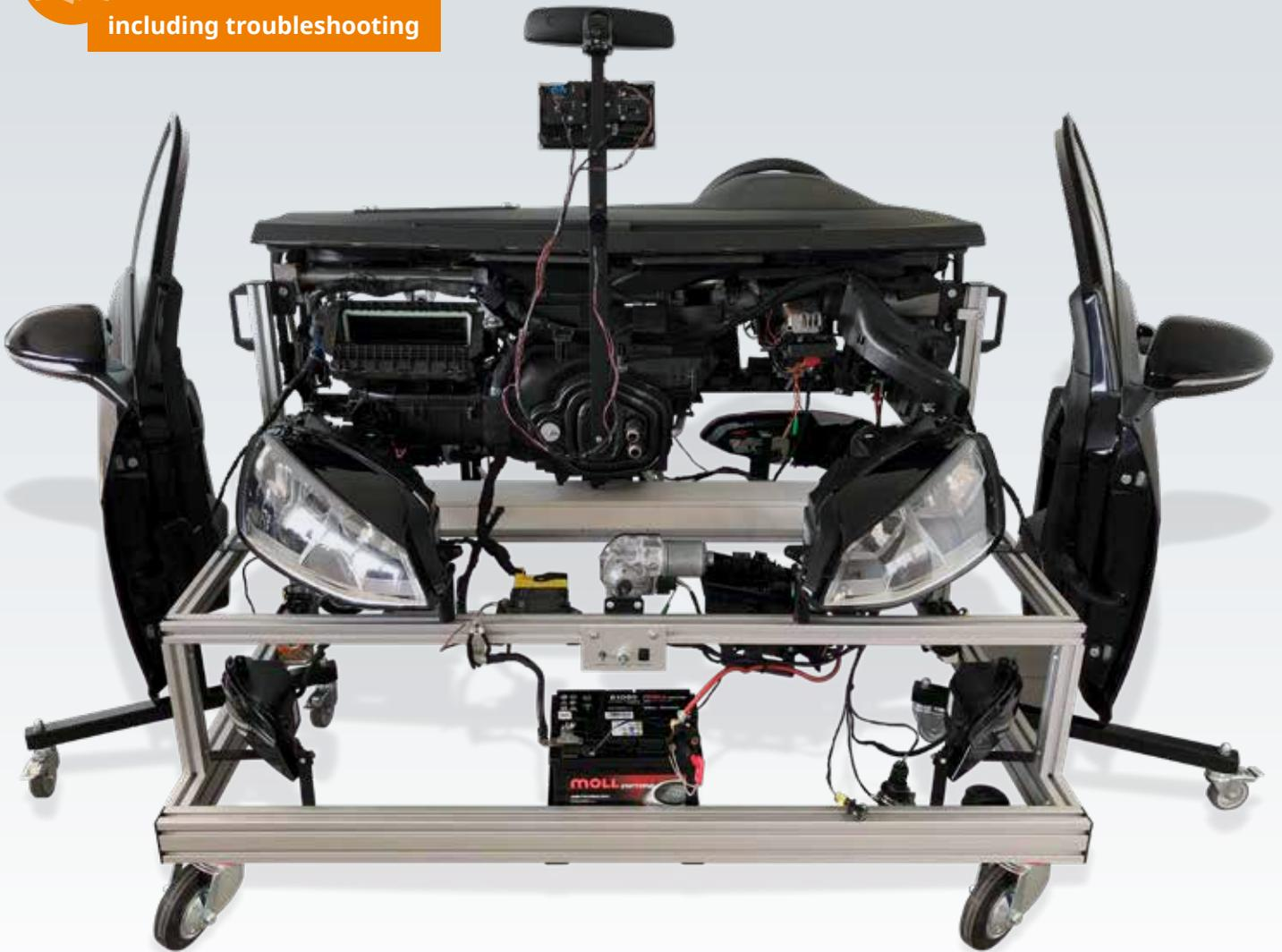
Carry out practical experiments using original components from a Volkswagen Golf 7, which is based on VW's MQB modular cross-component kits. This model for networked systems deals not only with the topics of actual CAN gateways but also covers the full electronic system for a steering column and includes fully functioning front doors with comfort controls.
