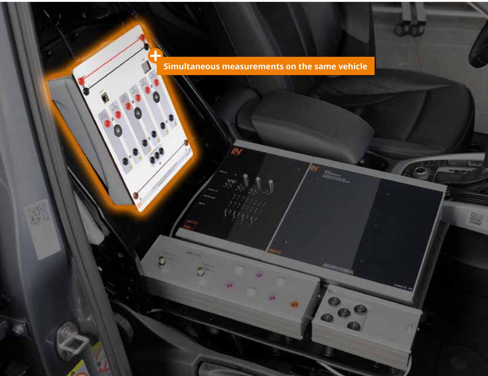
The measurement enhancement package makes it possible for multiple students to carry out measurements and diagnostics simultaneously on the same vehicle.
