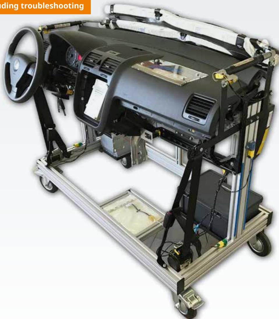
This training model provides all the necessary diagnostic skills with the help of a complete SRS system. It consists entirely of OEM components from a Volkswagen Golf 5, thus providing authentic learning experience. It also includes an on-board network control unit, original fuses and cable harness plus a full set of crash sensors. A full set of actuators is also provided, but these devices do not actually trigger so that it is possible to work with them safely.
