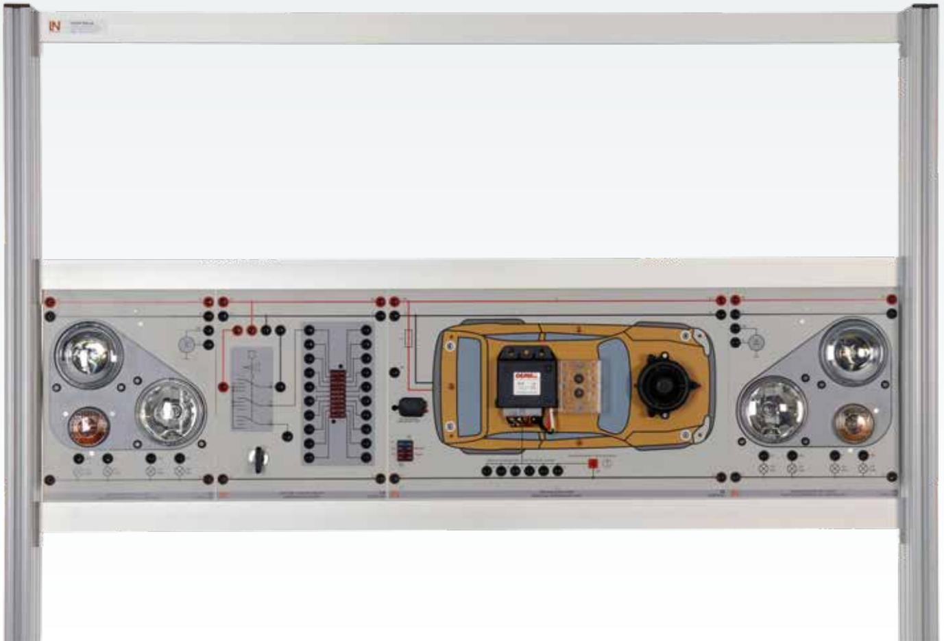
Alarm systems are such attention seekers. They may stay quiet and unobtrusive most of the time, but if unauthorised access or interference should be detected, all eyes and ears must be assailed by flashing lights and sirens. This modular system provides a fully functional alarm system, specially adapted for educational purposes and compactly laid out on a single board.
