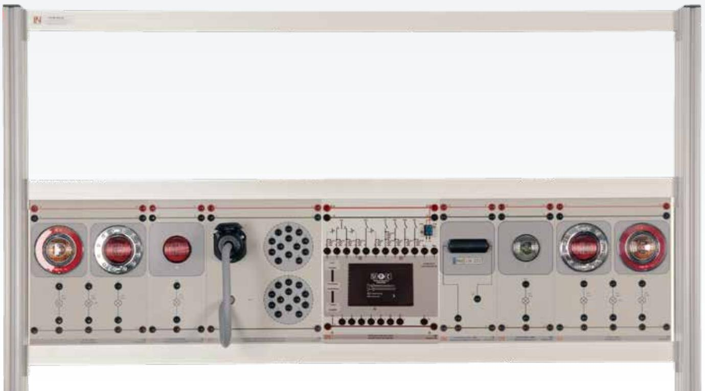
Teaching the topic of lighting for trailers has also become far more demanding in terms of the complexity of the electrical systems. The content imparted by the training system therefore goes beyond the principle of 7- or 13-pin plug connectors. It also explains how the towing vehicle is protected against overloading and when the control functions for the trailer meet regulations.
