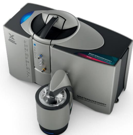
The Hydro MV is medium volume unit for the controlled, automated wet dispersion of samples for particle size analysis. Designed for applications that require smaller sample sizes, the Hydro MV is especially valuable when the supply of test material is limited or when dispersant usage must be minimized.
