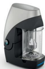
Hydro EV - A unique dip-in, semi-automated wet sample dispersion unit that can be used with 250 mL, 600 mL and 1000mL standard laboratory beakers.
