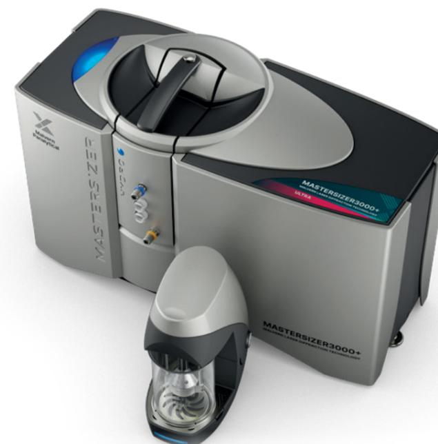
The Hydro EV has a unique dip-in centrifugal pump and stirrer design that achieves full and rapid dispersion in standard laboratory beakers, allowing close matching of the dispersant volume to the application requirements. Following measurement, the dispersion head can be raised out of the beaker, enabling quick cleaning and sample recovery.
