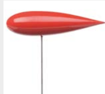
HM 170.08 Drag body streamlined shape length: 240 mm diameter: 60 mm
