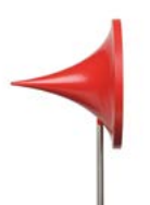
HM 170.11 Drag body concave shape length: 68,65 mm diameter: 80 mm
