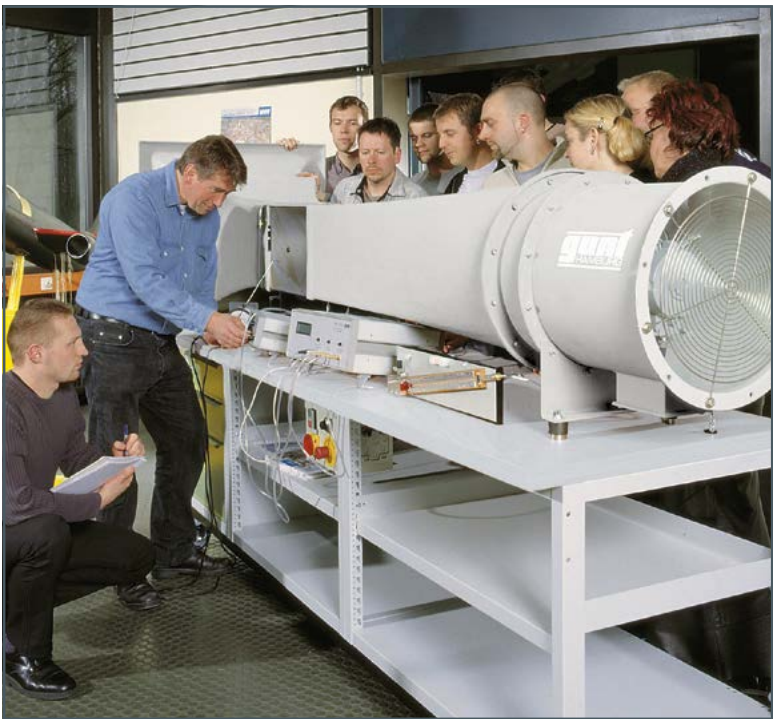
Training at the HM 170 Open wind tunnel at the Technical College for Aeronautical Engineering in Hamburg (Germany)
