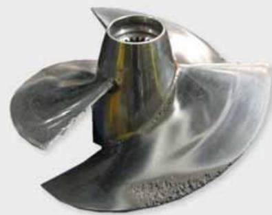
Ship's propeller destroyed by cavitation erosion
