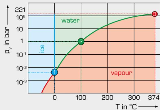
Temperature-pressure diagram of water
