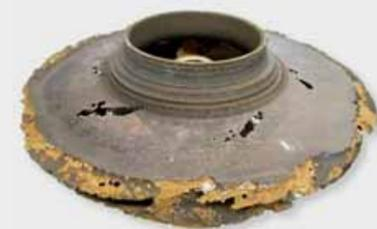
Pump impeller destroyed by cavitation erosion
