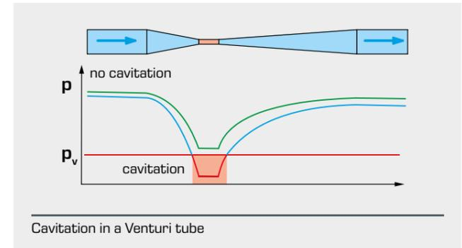
Cavitation in a Venturi tube
