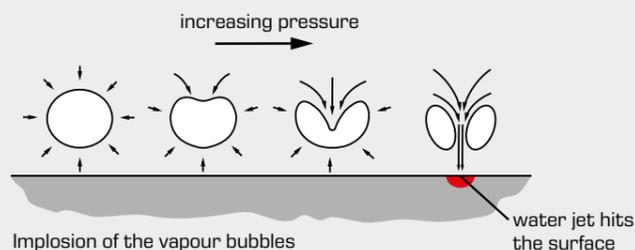
Implosion of the vapour bubbles
