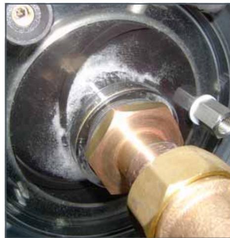
Formation of vapour bubbles due to cavitation at a pump impeller (HM 380)
