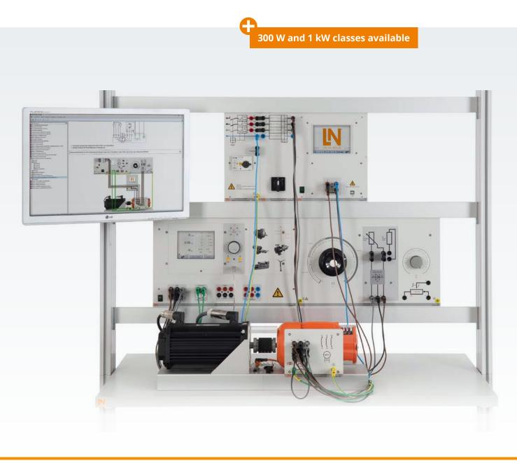
In contrast to squirrel-cage rotors, slip-ring rotors have a rotor equipped with wound coils. These can be connected to resistors or static converters via slip-rings. Speed adjustment is performed via these connection terminals.
