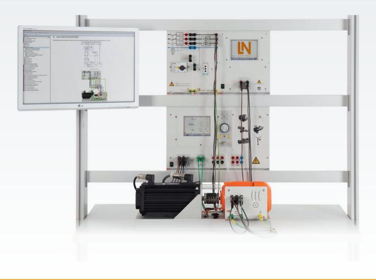
Smooth starters use phase-angle control to reduce the motor voltage during switch-on. The starting current drops proportionally to the terminal voltage. The power component of a smooth starter is usually comprised of two thyristors per phase switched antiparallel. To keep the power losses and the contingent heat arising from this as low as possible, the power semiconductors are shunted by an integrated power circuit-breaker subsequent to the start-up phase.
