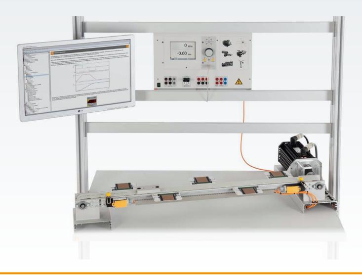
The focus of this training system is on practical hands-on learning of how modern positioning drives function and operate. The servo-machine testing system is operated as a positioning drive on a linear axis. Using software designed for education, students can explore hands-on how the positioning drive operates in the context of project work.
