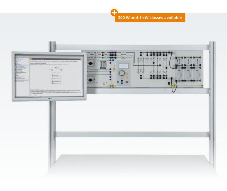
Line-commutated converters permit power to be fed from an AC or three-phase system to a DC circuit. These can be designed for operation in controlled mode using thyristors and triacs or uncontrolled mode using diodes.
