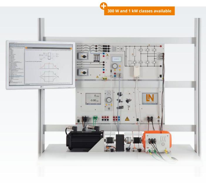
Three-phase drives are used today in almost all electrical drives. Mathematically the automatic control of such drives is both a complex and costly undertaking. The training system makes it possible to simulate sophisticated control algorithms with the aid of the special toolbox for Matlab<sup>®</sup>/ Simulink<sup>®</sup> and subsequently test them by means of automatically generated code on real intrinsically safe hardware incorporating a motor and load.
