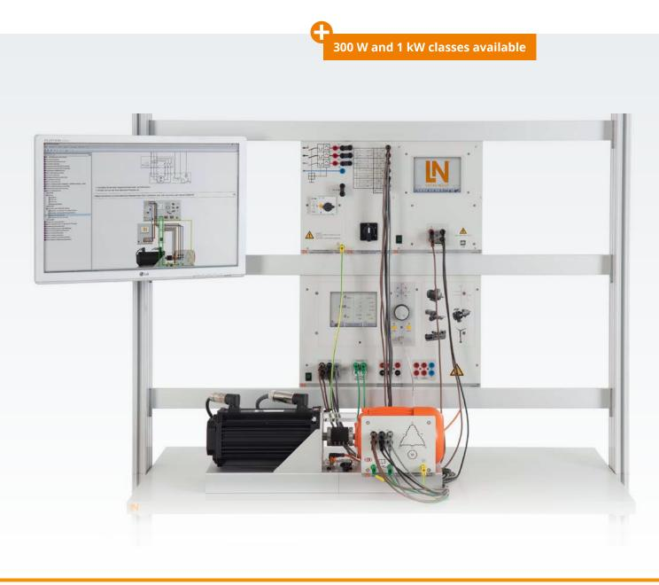
Thanks to its special winding, the three-phase motor with Dahlender circuit is able to operate the motor with squirrelcage rotor at two different speeds. The ratio of speeds is 2:1 for this circuit. With this motor type, simple drives can be designed with two speeds, for example, a two-staged ventilator drive.
