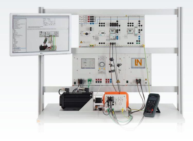
Squirrel-cage motors are designed to operate at constant load. Changes in the load state but also high starting currents can lead to the impermissible and excessive overheating of the motor. Sensors monitor the motor's temperature and current consumption. They activate protective circuitry like motor circuit-breakers, motor protective relays or thermistor relays.
