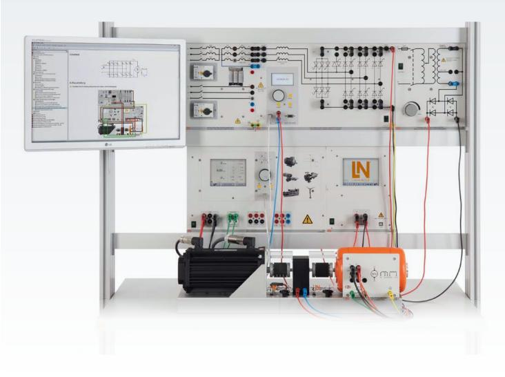
Variable-speed DC drives excel thanks to their very good speed and torque controllability and extremely high dynamic response. When it comes to power semiconductors operating with large-scale drives at high power levels, one resorts to line-commutated converters with thyristors. These components stand out because of their capacity to handle overload and their low tendency for power losses.
