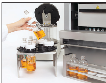
Sample transfer from SpeedExtractor to Multivapor™
