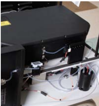
Hermetically sealed spectrometer eliminates frequent desiccant regeneration.
