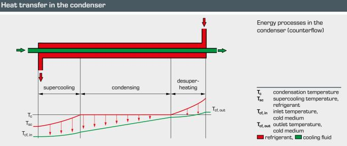
The energy processes in a properly designed condenser can be assigned to three different areas.
