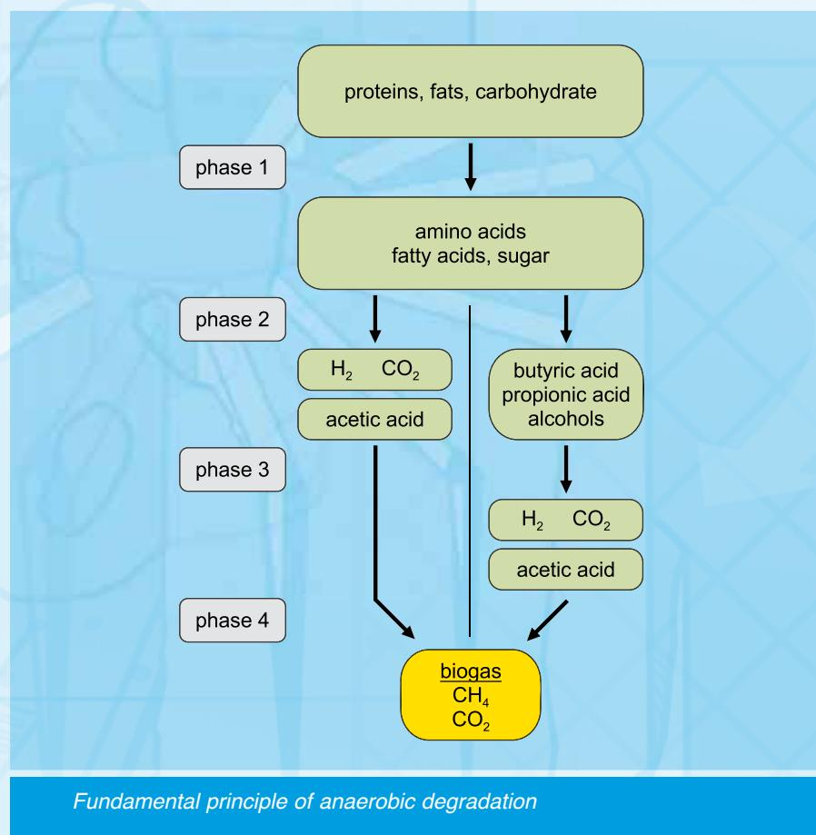
Fundamental principle of anaerobic degradation
