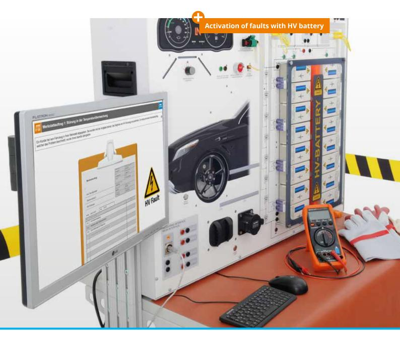
Diagnostics of faults which can be specifically activated allows students to gain skills which will be of use to them in a real vehicle workshop.
