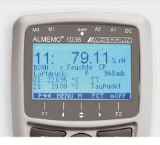
Reference measuring instruments for humidity and temperature **High-precision measurement** with the Pt100 psychrometer and Pt100 sensors Resolution Temperature 0.001 K Relative humidity 0.01 % Dew point 0.01 K
