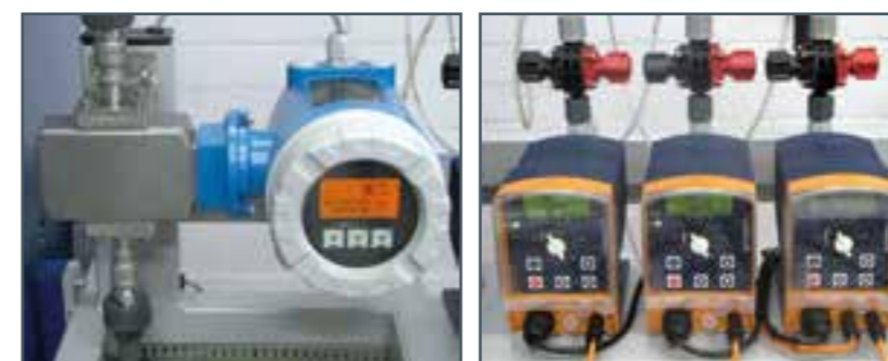
Standard at GUNT: use of high-quality industrial components such as professional metering pumps and electromagnetic flow meters
