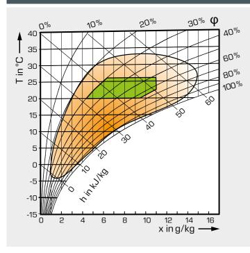
In the h-x diagram temperature **T**, enthalpy **h** and relative humidity  $\phi$  are plotted above the absolute humidity x.
