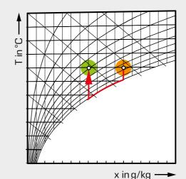
Cooling to 100% r.h. (saturation), condensation of the humidity on cold surfaces. Followed by heating to the desired temperature.
