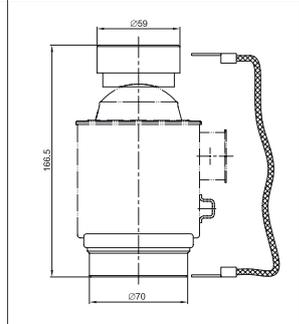
Truck scale load cell PR 6221 with standard load disc kit PR 6021/00N
