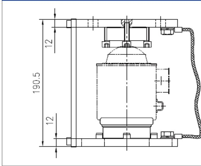
Truck scale load cell PR 6221 in mounting kit PR 6021/01N
