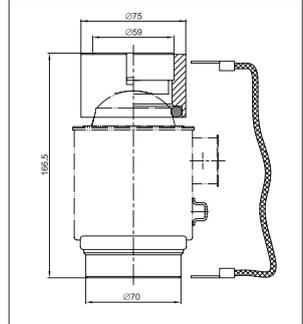
Truck scale load cell PR 6221 with turbo load disc .. /04N
