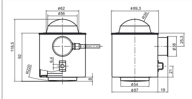
Truck scale load cell PR 6221
