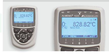
Reference measuring instrument for temperature High-precision measuring by means of thermocouples Types N, S, R, B Resolution 0.01 K, up to 1800 °C
