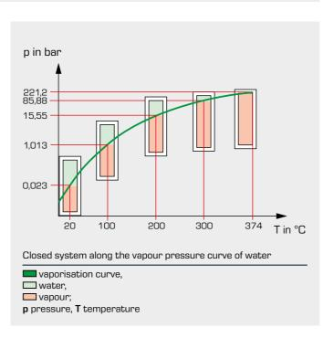
In a closed system filled with liquid, a thermodynamic equilibration sets in between the liquid and its vaporised phase. This state is called the saturation state. The prevailing pressure is referred to as vapour pressure, in case of water steam pressure or saturated steam pressure, and the temperature is known as saturation temperature. The vapour pressure curve can be derived from both. This curve is shown in the phase diagram of water.
