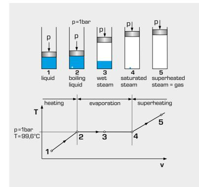
Evaporation of water: change of state when heating water under constant pressure **p** = 1 bar
