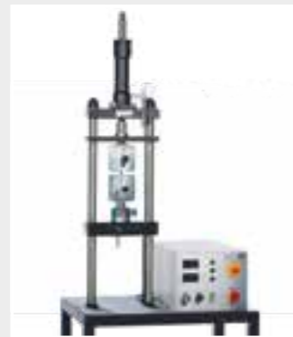
The WP 310 experimental unit generates a 50kN test load
