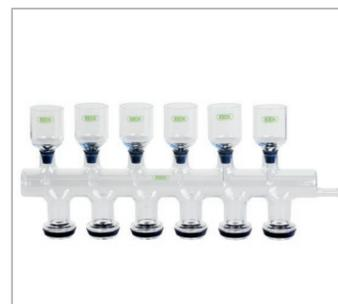
Use dedicated suction modules for aqueous samples (condensate trap), accelerated digestion ( $H_2O_2$ ), metal or COD digestion (reflux).
