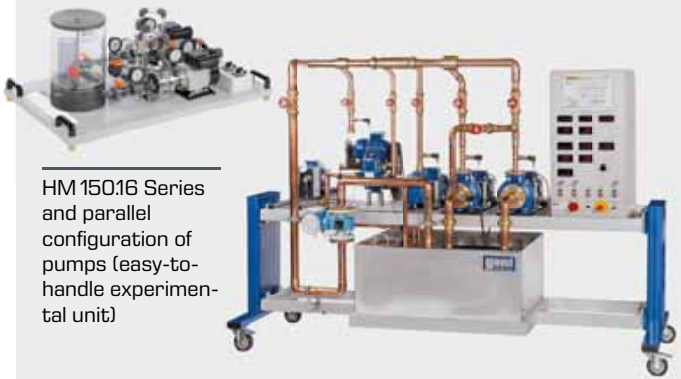
HM 362 Comparison of pumps (complex trainer)
