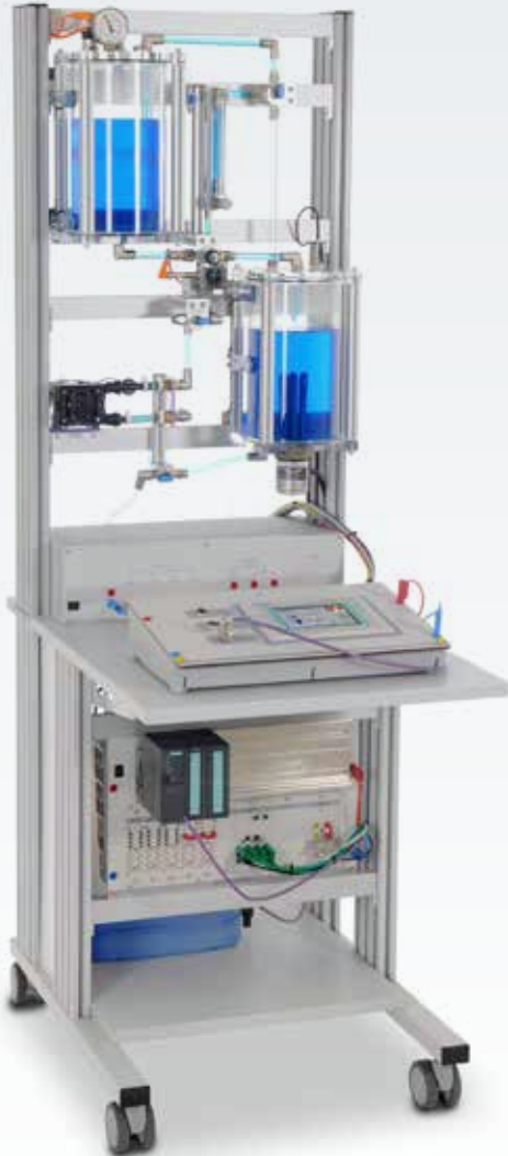
IPA 1 Compact Station, Control of Process Variables via PLC
