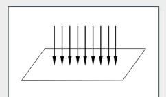
Linear force / line load: continuously distributed force along a line (idealisation in mechanics)
