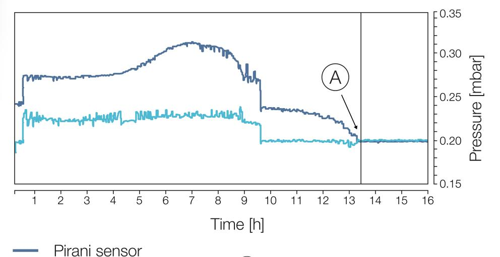
Pressure measured by pirani and capacitive sensor for manifold application with round bottom flasks containing 5 wt% mannitol.
