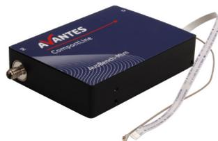
Our miniature bench, the AvaBench-75-MN (CompactLine) features a Czerny-Turner design with a fiber-optic entrance connector (SMA), collimating focusing mirrors and a diffraction grating.
