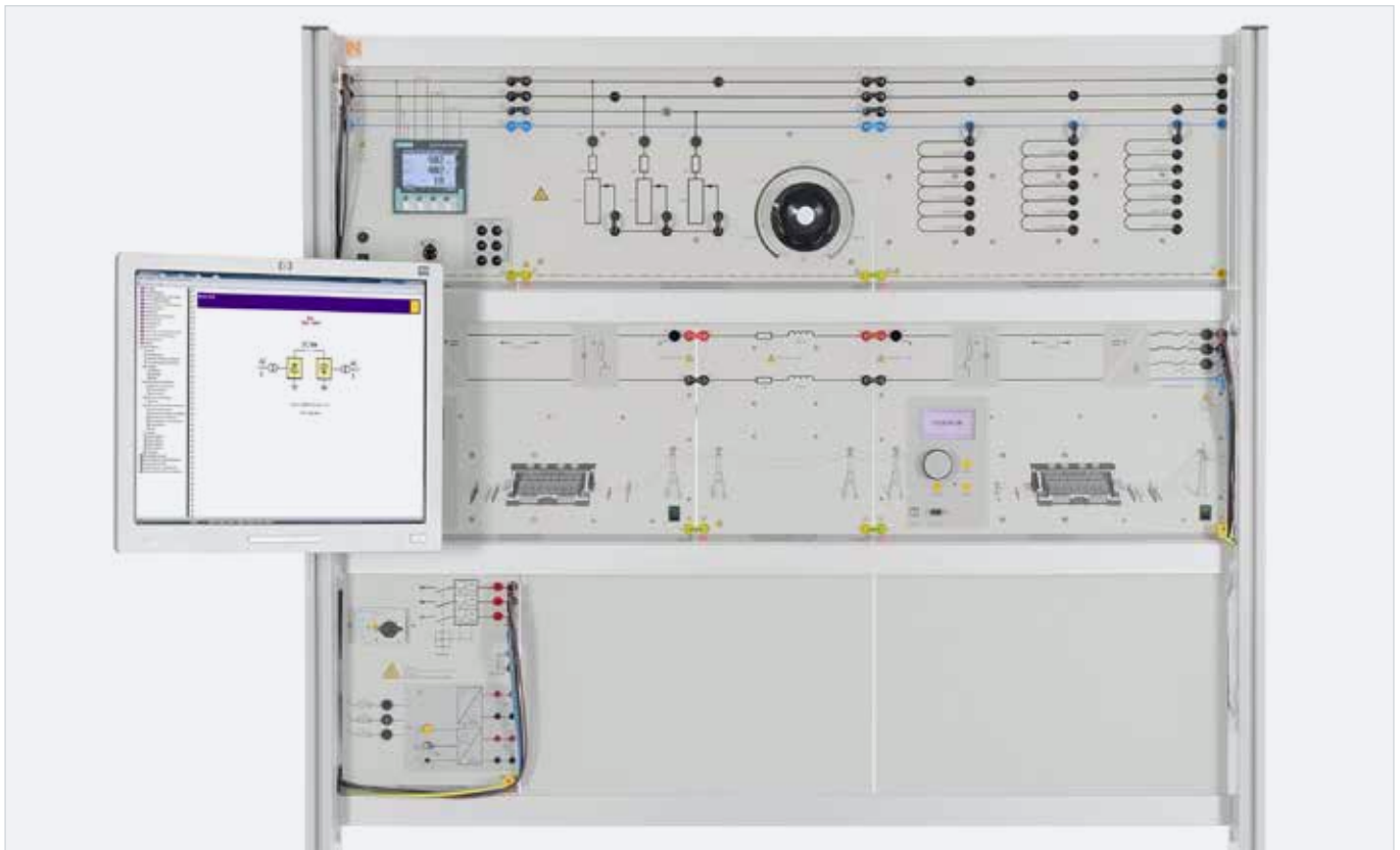
Experiment example "High voltage DC transmission" EDC1
