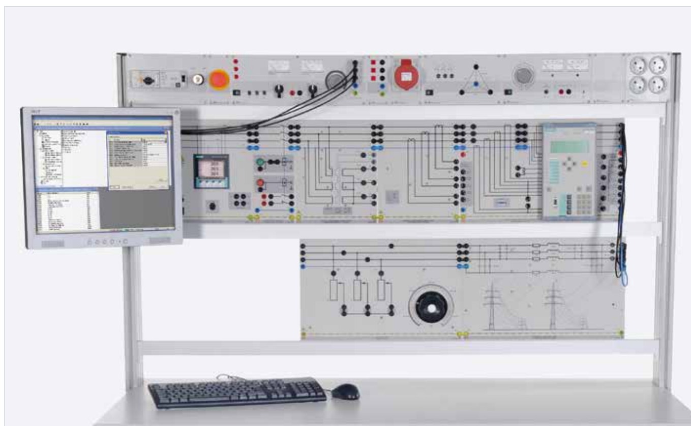
Sample experiment "High-speed distance protection" ELP 7
