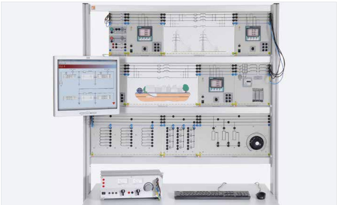
Sample experiment „Investigations on interconnected network grids with cables and overhead lines“ EUL 6
