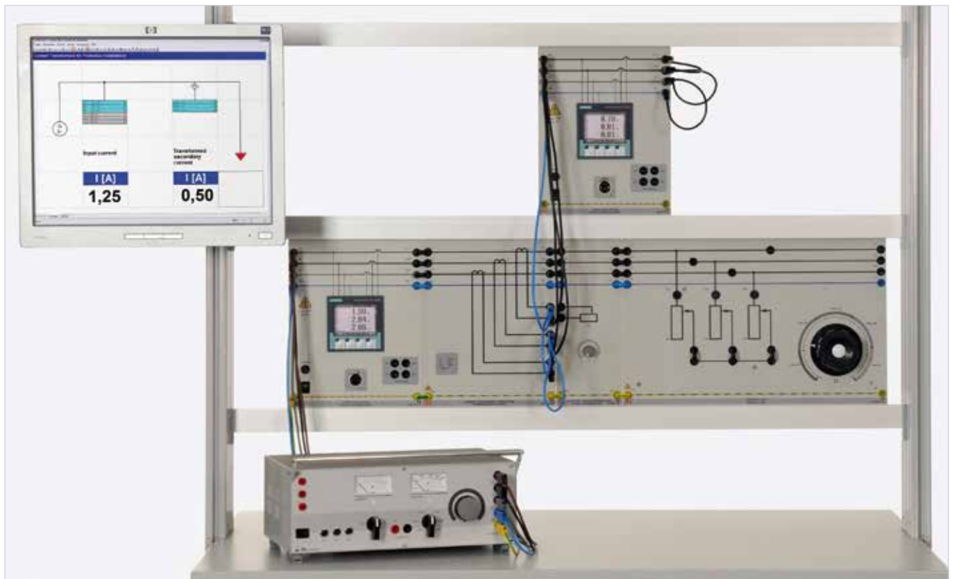
Sample experiment "Current transformer" EUB 1
