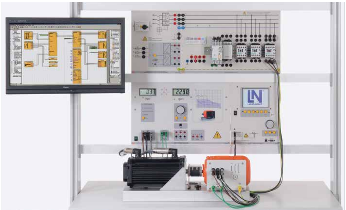
Sample experiment "Motor management relay" EDT 51
