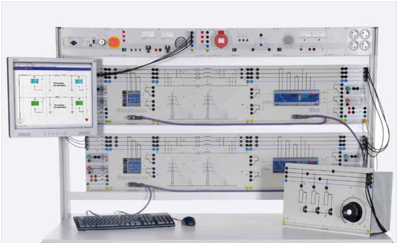
Sample experiment "Protection of parallel lines" ELP 6
