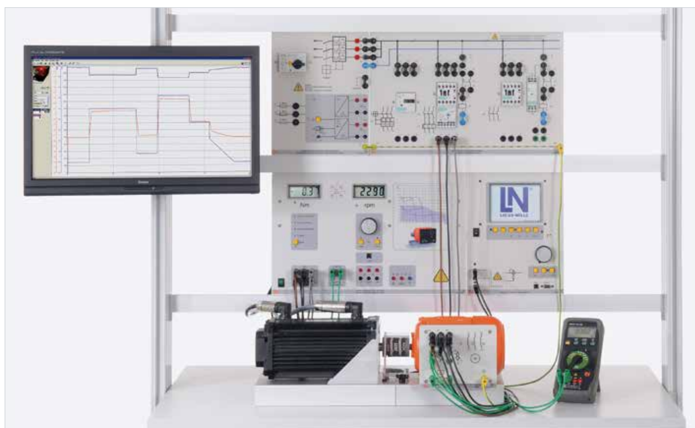
Sample experiment "Protection of electric machines" EEM 4.6
