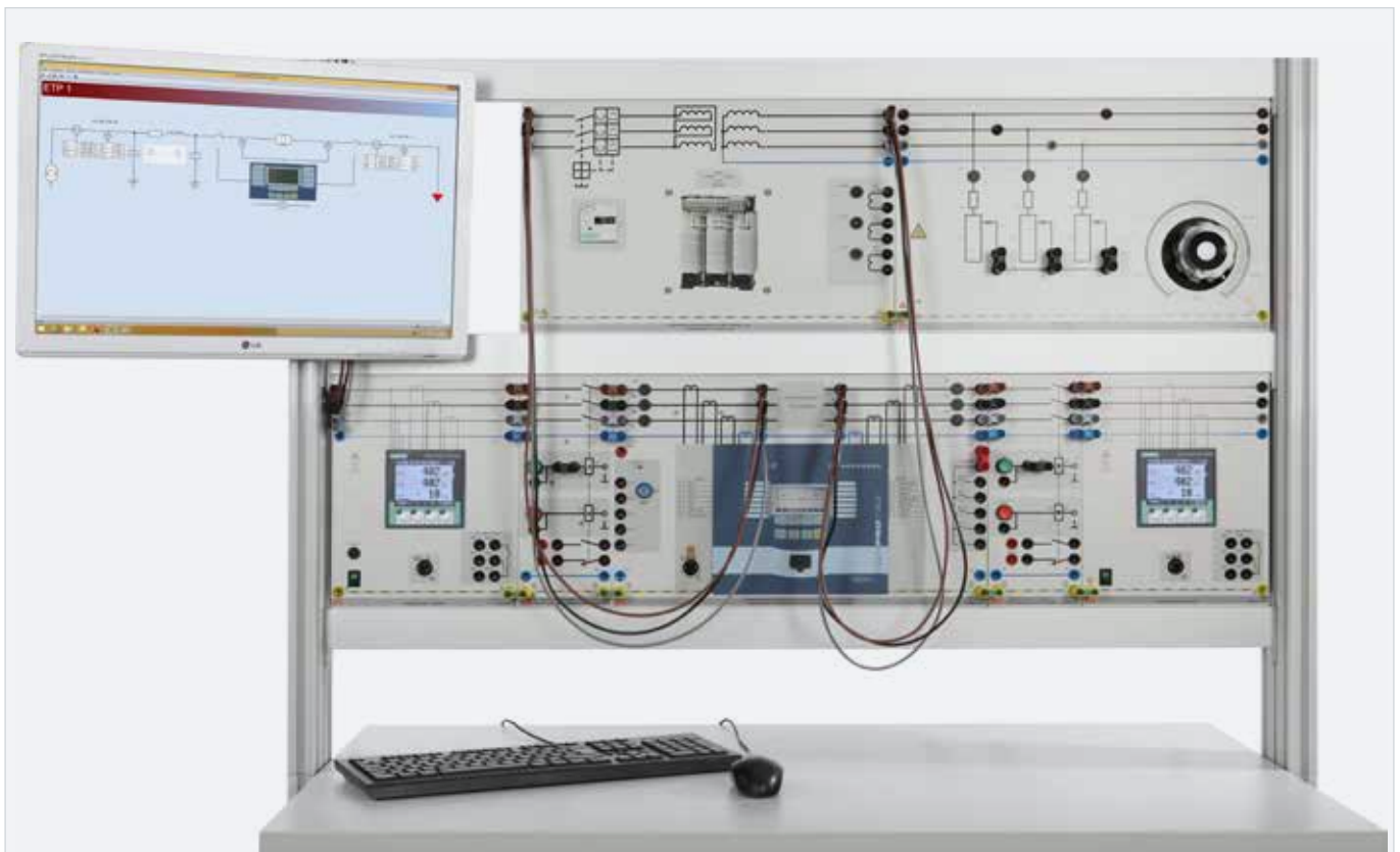
Sample experiment "Time overcurrent protection" ETP 2
