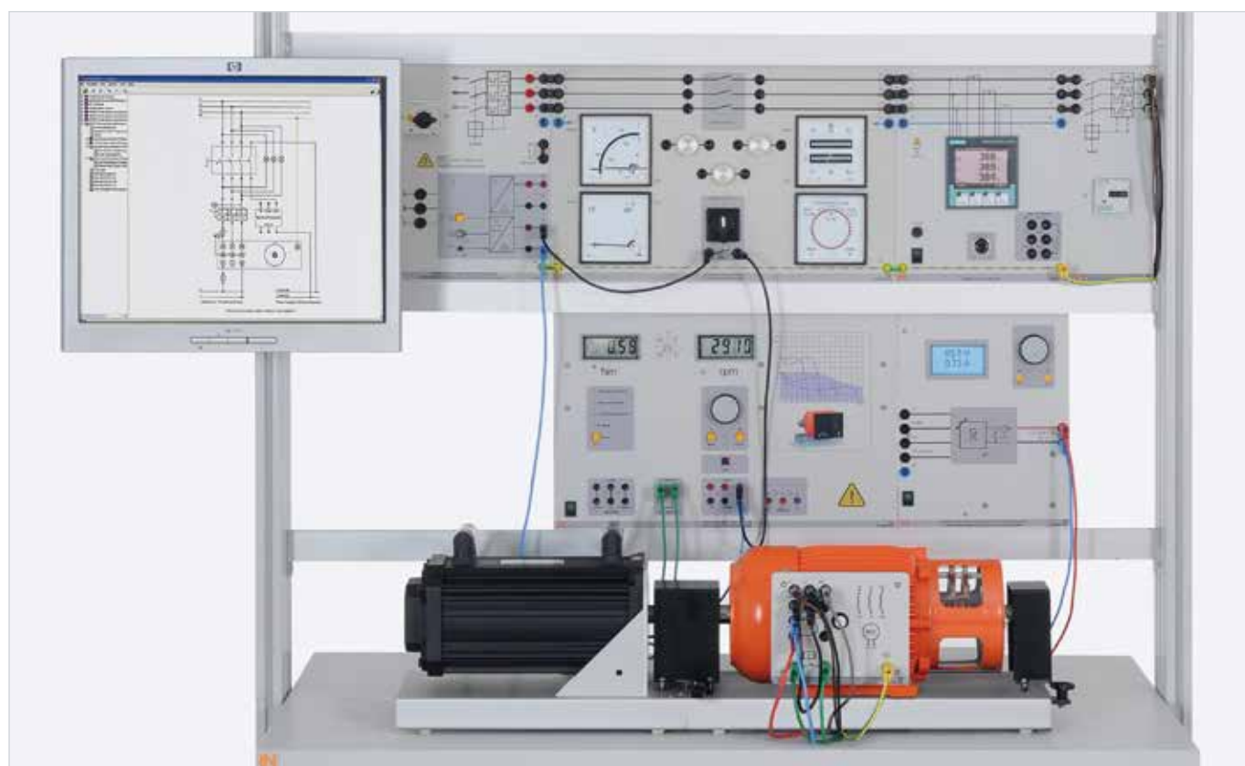
Sample experiment "Manually operated synchronising circuits" EUG 1
