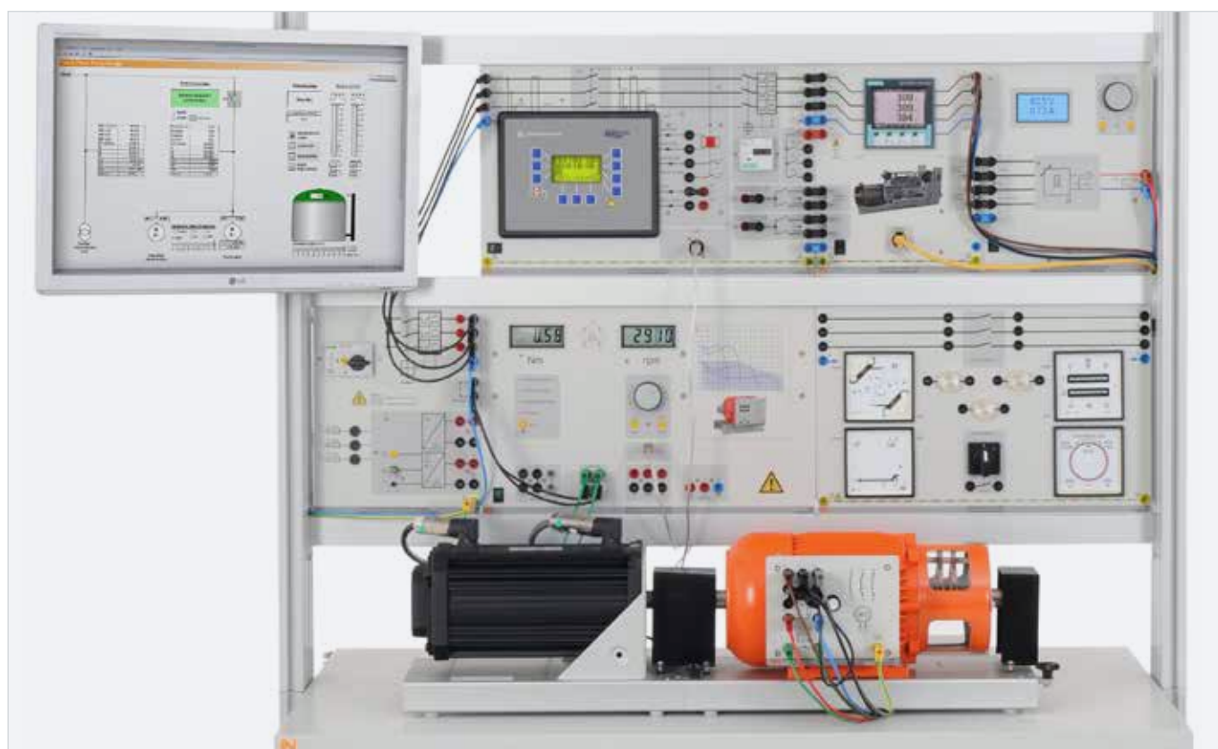
Sample experiment "Generator protection" EGP 1
