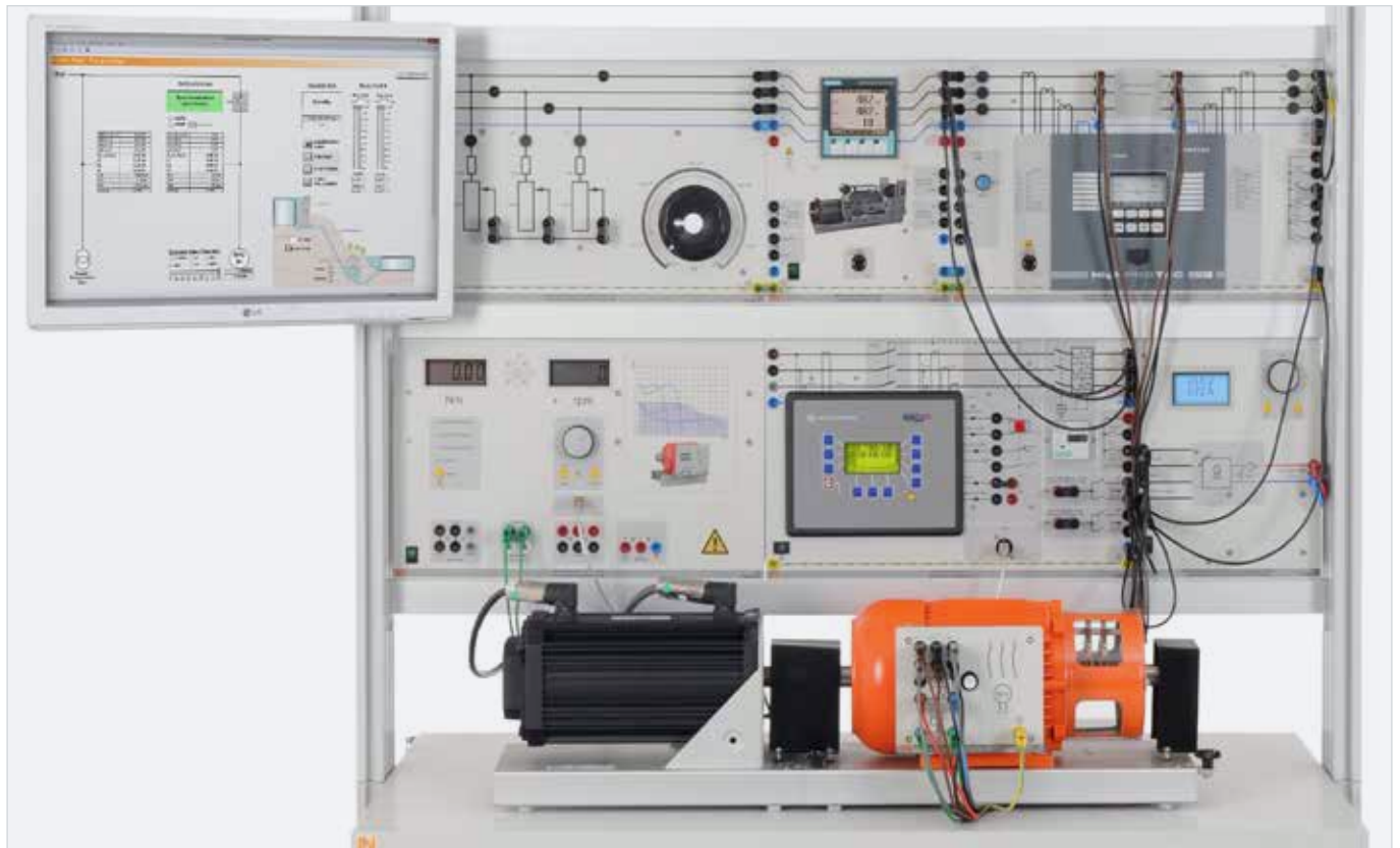
"Generator differential protection" EGP 2
