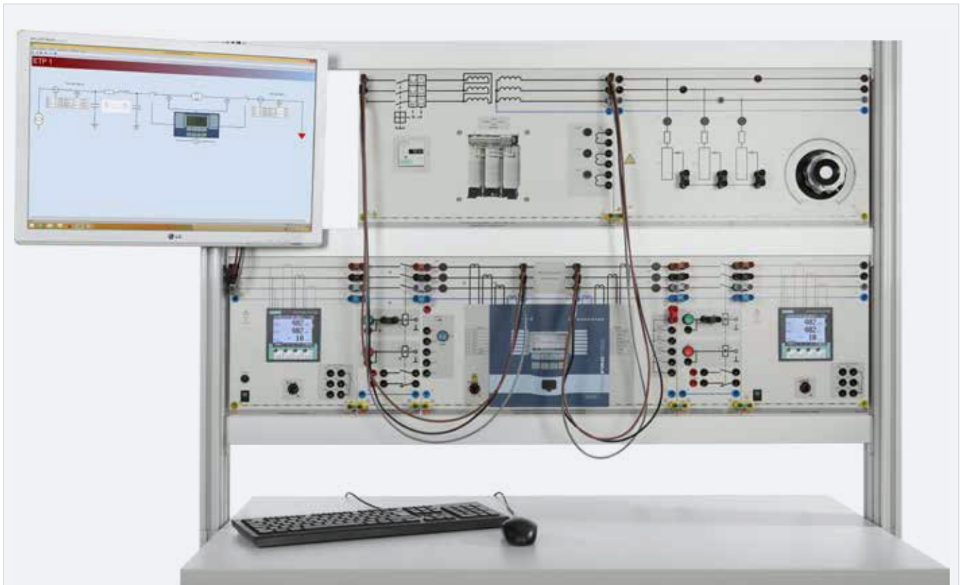
Sample experiment "Transformer differential protection" ETP 1
