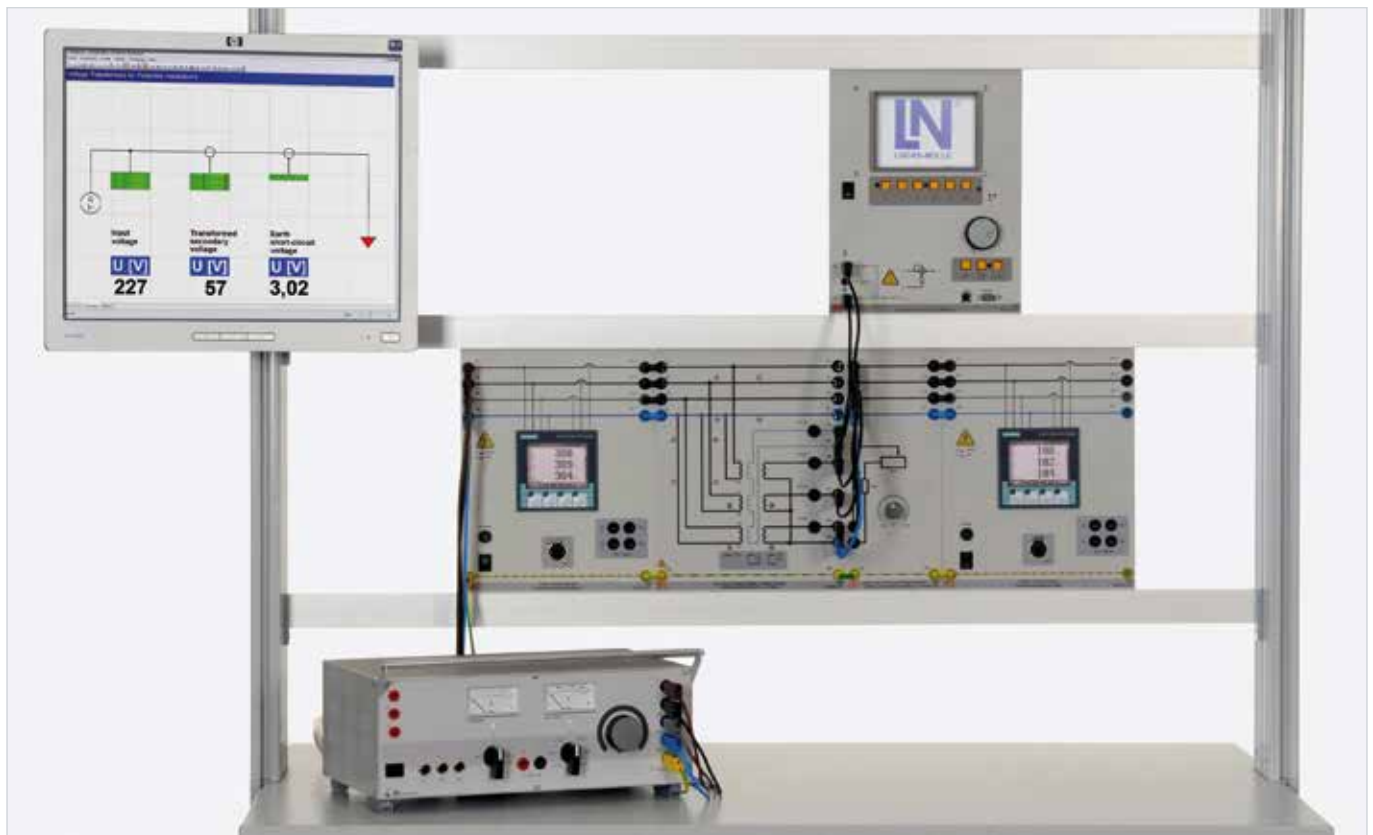
Sample experiment "Voltage transformer" EUB 2
