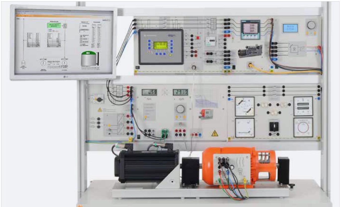
Sample experiment "Automatic synchronising circuits" EUG 2
