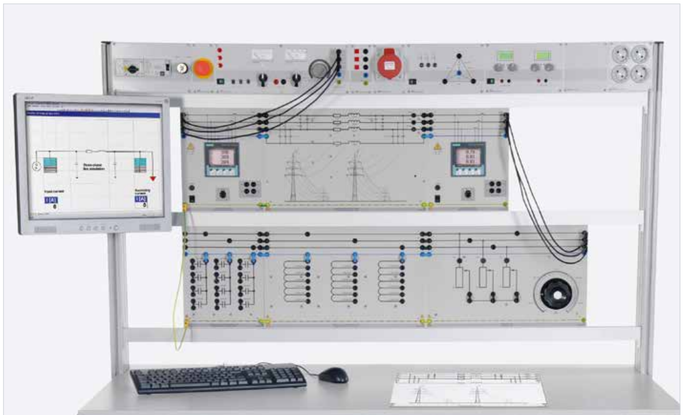
Sample experiment "Investigations on three-phase lines" EUL 1
