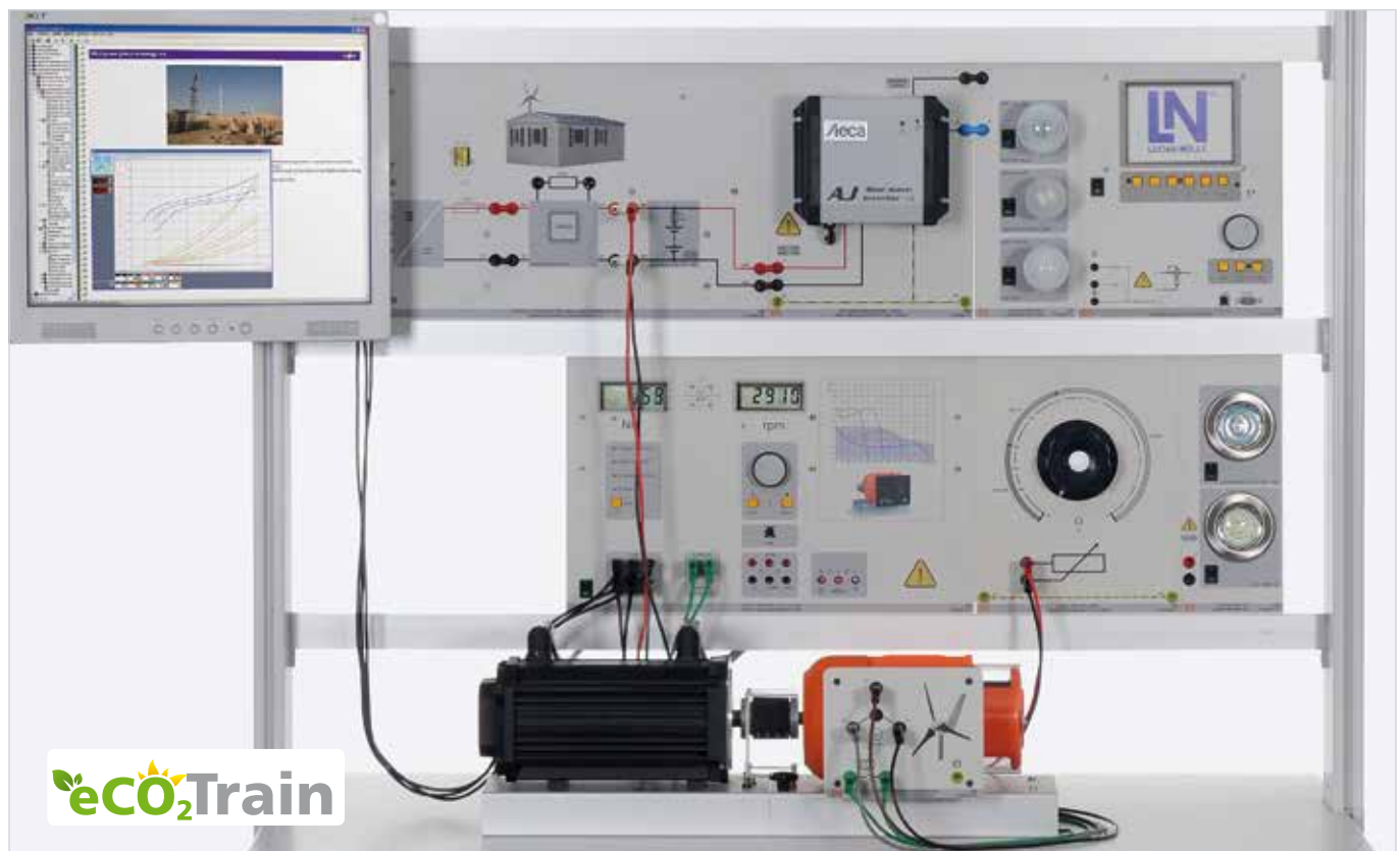
Sample experiment "Small wind power plant" EWG 2
